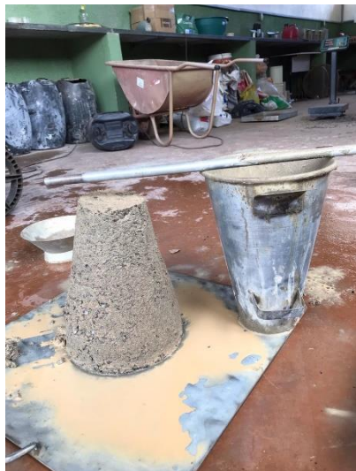
Figura – 6 Slump test do CRF2
